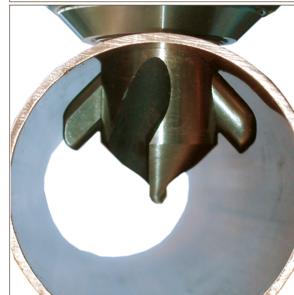
Figure 13.6: Extending the forming pins inside the run tube
