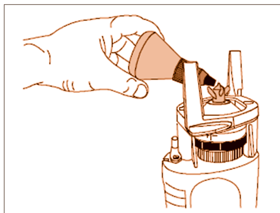
Figure 13.3: Lubricating the drill head
