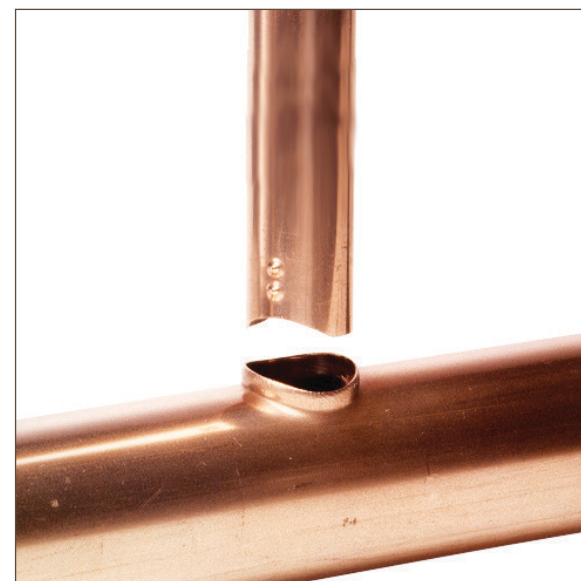
Figure 13.11. Aligning the dimples with the run of the tube
