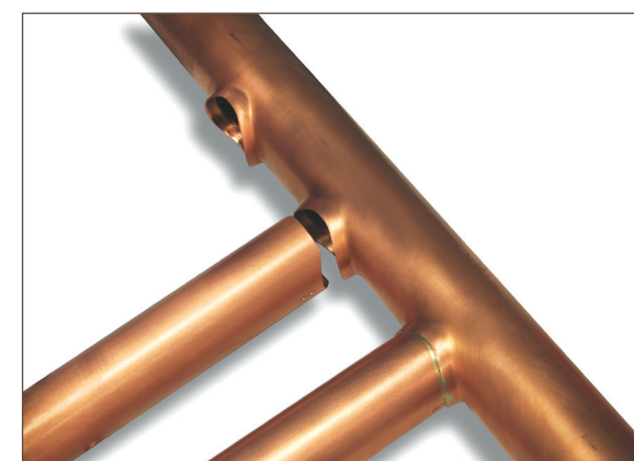
Figure 13.1. Mechanically formed extruded outlet requires only one brazed joint
