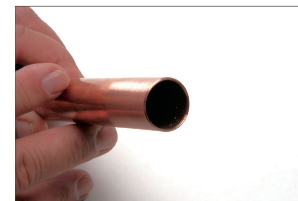
Figure 13.8. Reamed and deburred branch tube end
