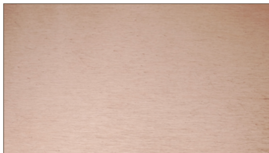
Figure 3.1C. Directionally textured example: C11000, brush finished.
