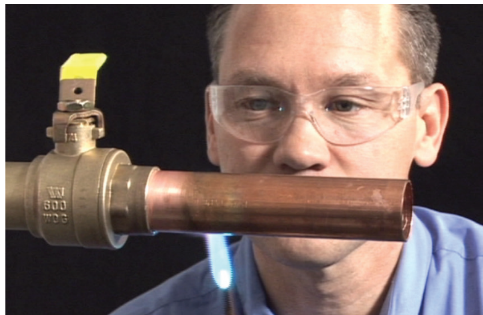
Andy Kireta Jr. demonstrates proper soldering. Photo Credit: Copper Development Association
