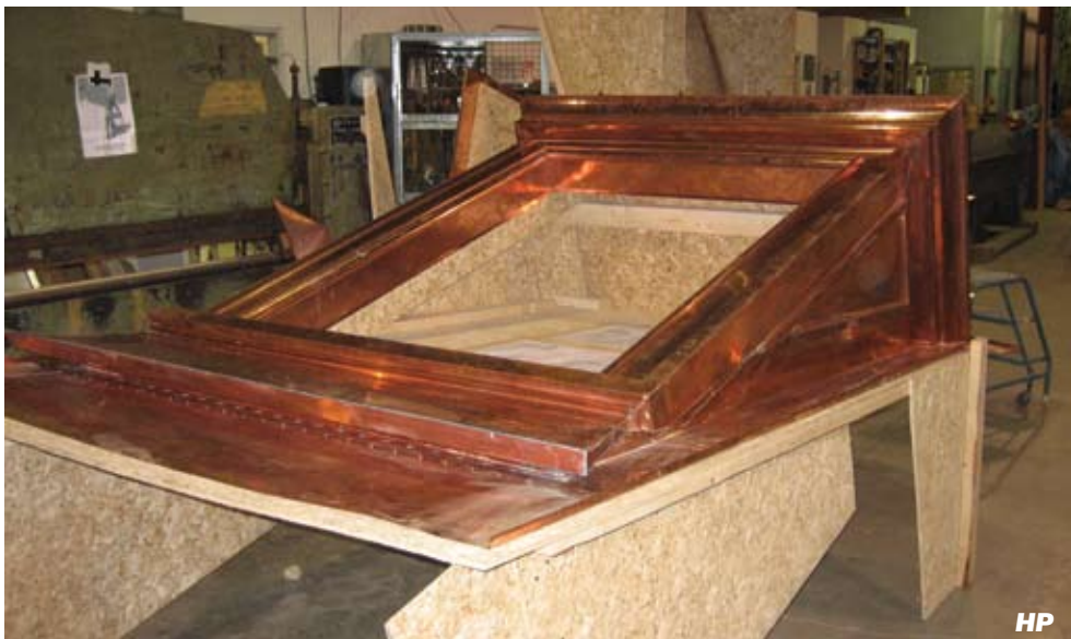
A new copper dormer being fabricated for the Plaza Hotel in New York.
