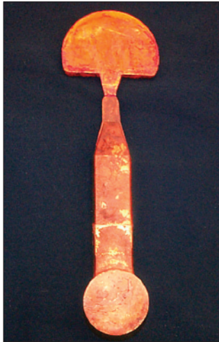
Fig. 3 – Test casting used to evaluate and compare candidate mold materials. A two pound copper biscuit is above the gate area and runner bar.
