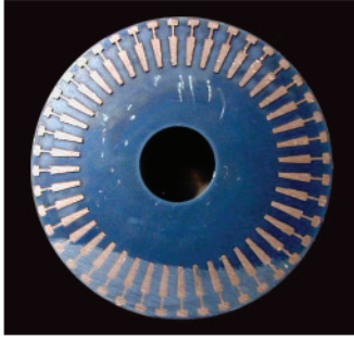
Fig. 9 – Cross-section of rotor showing copper filling the slot openings by the pressure.
