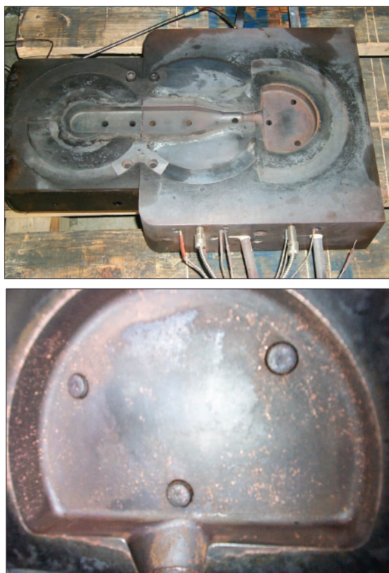
Fig. 6 – Top: Moving half TZM and Anviloy die inserts after 940 shots. TZM is in the bottom (left) position and Anviloy in the middle and upper positions. Electrical resistance heaters and thermocouple leads are visible on the lower edge of the mounting plate. Bottom: Close-up of Anviloy die inserts after 500 shots.
