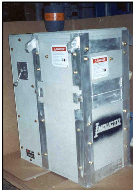
Figure 7. One section of the die set purchased from Buhler for die casting copper rotors.
