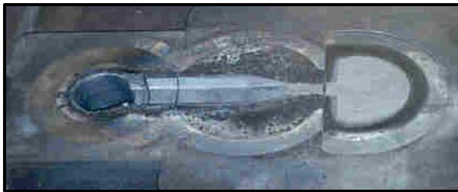
Figure 6. Fixed die half with Inconel alloy die inserts after 300 shots. The dies have oxidized a little but have not cracked after 380 shots.
