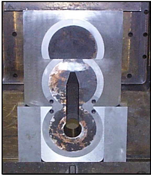
Figure 3. The H-133 steel test cavity tool set after the first several shots.
