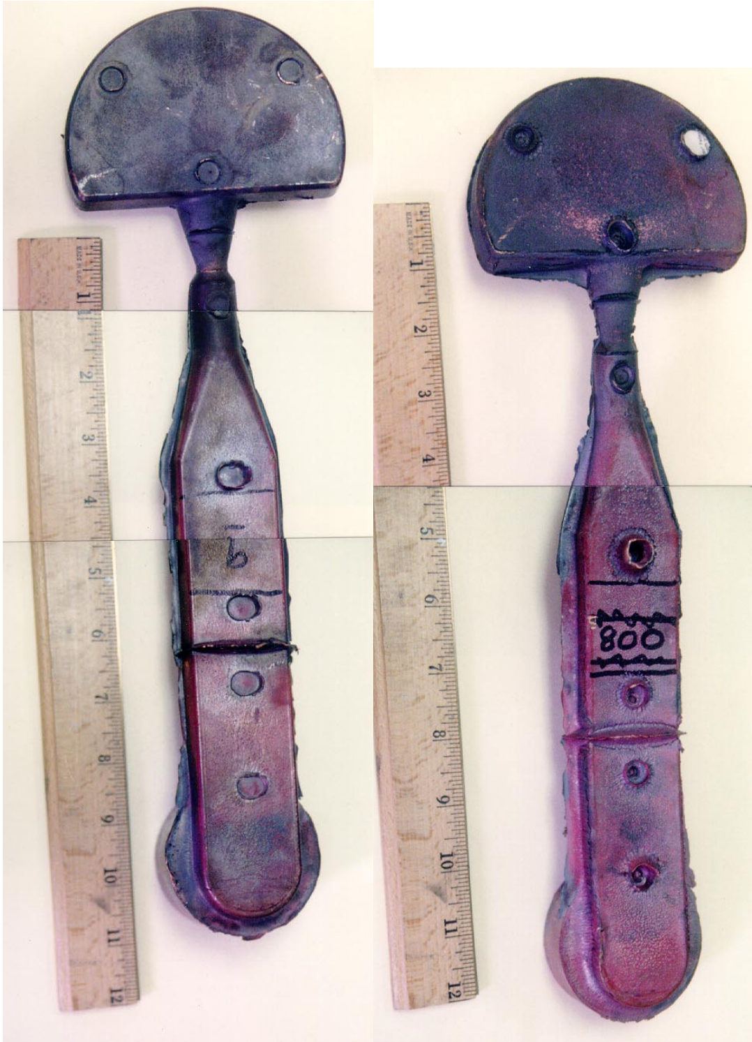
Figure 3. Comparison of die-casting shot numbers 9 (left) and 800 (right). Some degradation of the H-13 steel die inserts is evident from the increased width of the flash between inserts and by the erosion at the gate area.
