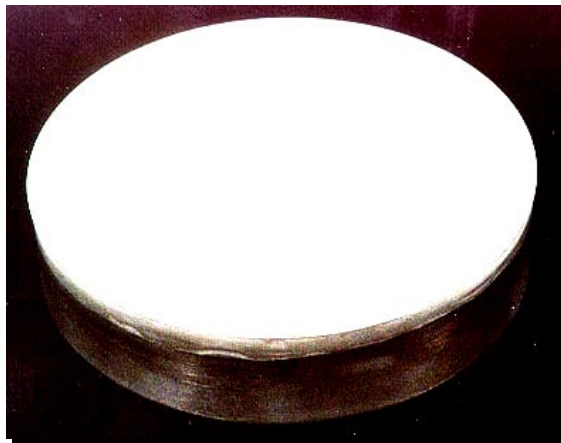
Figure 7. Tungsten chemically vapor deposited (CVD) onto a molybdenum substrate by the ThermoTrex Corporation.
