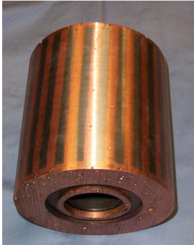
Figure 8 – Photograph of Copper Rotor Turned on the OD to Expose the Conductor Bars. Trapped air bubbles are not seen in the bars but are clearly visible in the end ring.
