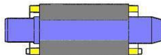
Figure 3 – Schematic Diagram of Heated Nickel-Base Alloy Dies for Rotor Die Casting. The arbor (dark blue) and the steel laminations (dark grey) are shown as assembled in the insert
