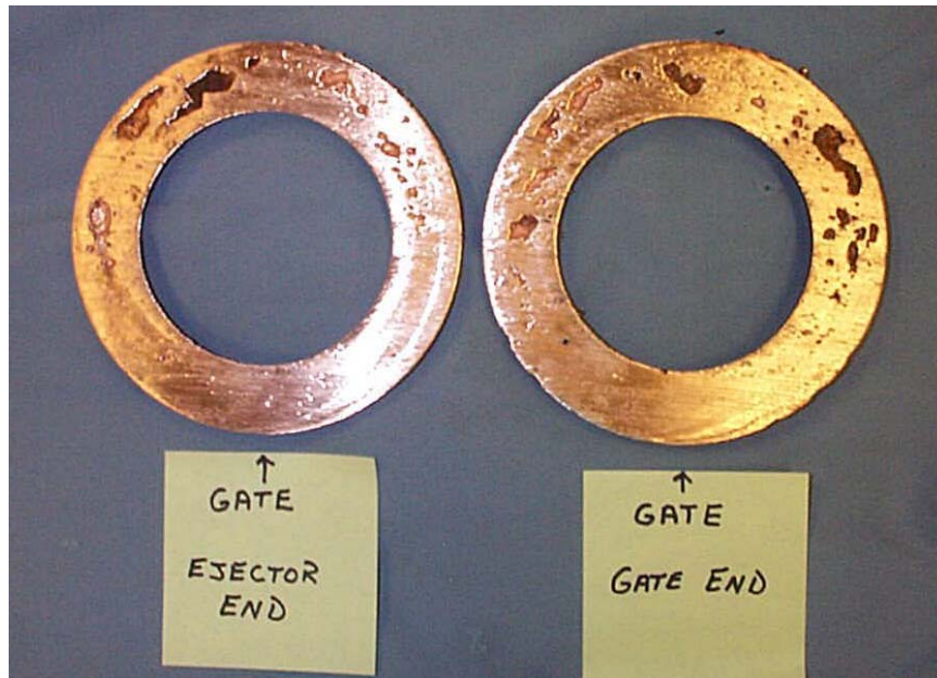
Figure 5 - Photographs of Sectioned End Rings from Copper Rotors Typical of Baseline Casting Conditions.
