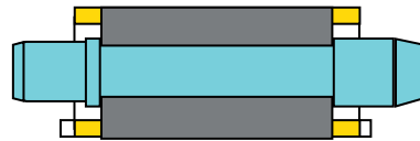
Fig. 12 – Horizontal pressure die caster with tooling for rotor casting in closed position. The arbor (dark blue) and the steel rotor laminations (dark gray) are shown in the insert and in position in the machine. Copper from the shot sleeve biscuit, runner bar and end rings is shown in yellow. The nickel alloy and ring inserts are shown in medium blue with electrical resistance heater elements in red. These are backed with insulation (pink) as are the runner inserts, which would be nickel alloy or tungsten. Red circles here indicate heater positions. The moveable slide to allow insertion and removal of the rotor is shown in green. Ordinary steel backing plate of the master mold set are shown in light gray. (Courtesy of DieTec, GmbH).
