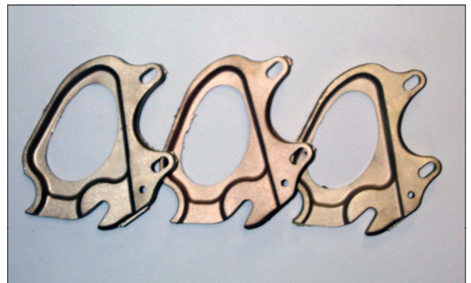
Fig. 14 – A part produced in three copper alloys by die casting SSM-processed billet.
