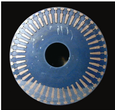
Fig. 13 – Cross-section of rotor for 3-phase motor showing copper filling the conductor bar shots.
