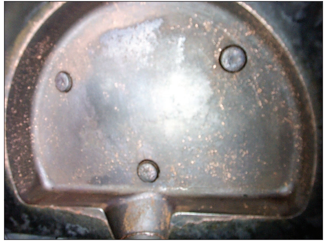
Fig. 10 – Left–Moving half of TZM and Anviloy die inserts after 940 shots. TZM is in the bottom (left) position and Anviloy in the middle and upper positions. Right–Close up of Anviloy die insert after 500 shots.
