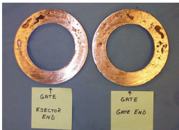
Fig. 3 - Photographs of sectioned end rings from copper rotors typical of baseline die casting conditions.
