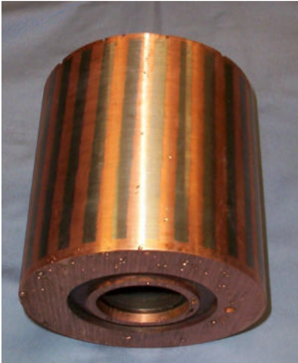
Fig. 6 - Photograph of copper rotor turned on the OD to expose the conductor bars. Trapped air bubbles are not seen in the bars but are clearly visible in the end ring.
