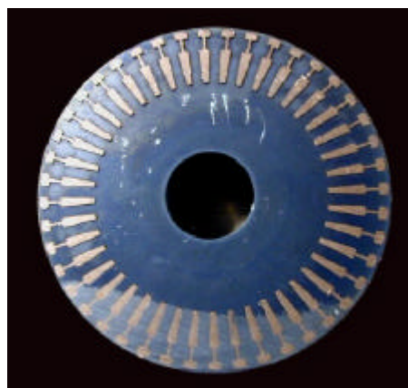
Fig. 2 - Cross-section of rotor for three-phase motor showing copper filling the conductor bar slots.
