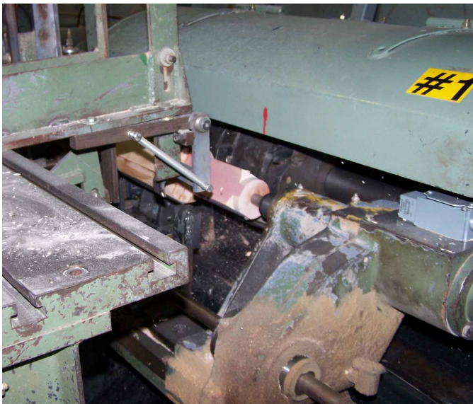
Figure 1. A rough-turned bowling pin and the built-up billet from which it is made. Turning is only one of many energy-intensive steps in the pin's manufacture.
