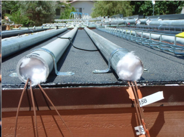
Fig. 5 – Cotton Used to Close Ends of Wireways
