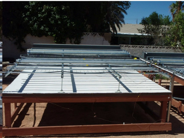
Fig. 3 – Samples Mounted 12 Inches off White Roof
