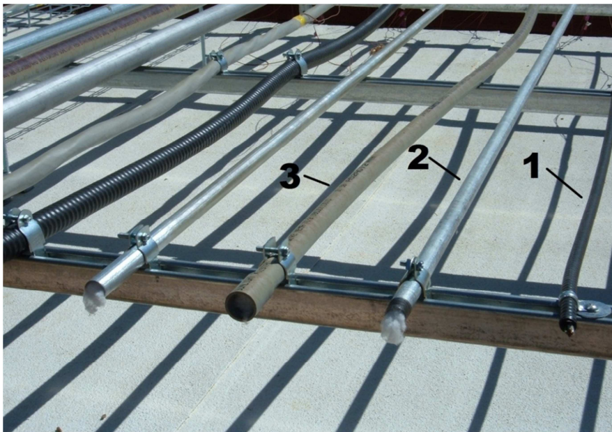
Fig. A1 – No. 12 MC (1), \frac{1}{2} RMC (2), \frac{3}{4} PVC (3)
