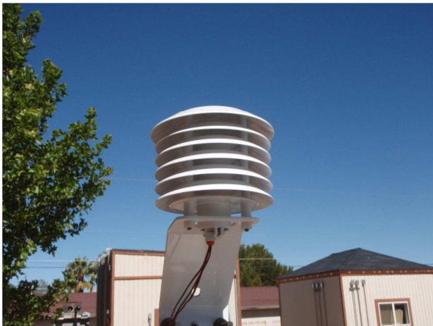
Fig. 6 – Aspirated Enclosure for Outdoor Temperature
